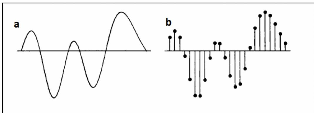
**Figure 26.** Converting an audio signal into a discrete signal
