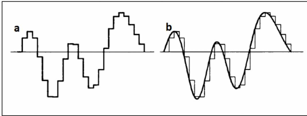
**Figure 27.** Conversion of a discrete signal into an audio signal
